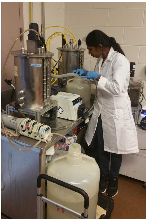
Figure 1: MS student Brindha Murugesan (University of Cincinnati) is optimizing a bench-scale membrane bioreactor system with the carbon nanotube composite membrane.
