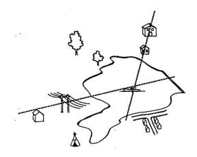
The lake monitor in this illustration is triangulating his position by lining up the tops of two houses in one direction with the line-up of the house and power poles in the other. When all four objects are in line, the monitor is over the sampling site.
